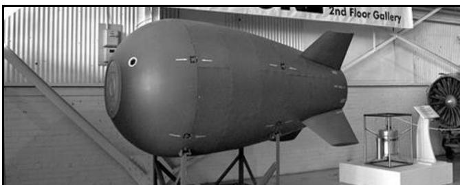
The bomb was blimp-like in its design – 3.25 meters long and 1.5 meters wide. It weighed five tons. According to the United States Air Force (USAF,) the bomb did not contain the plutonium core necessary for a nuclear detonation.
